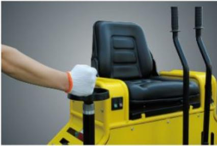
Foldable wheel controls make a convenient and ergonomical adjustment on the blade pitch
